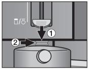
Press the steam lever, 1, down to connect the valve with the cappuccinatore, 2.
